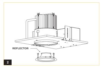
Separate REFLECTOR from fixture.
