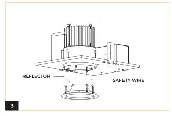
Make power connections. See Circuit Diagram below. Connect safety wire and push reflector into frame ensuring the trim is flush to the ceiling.
