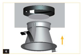
A. Place the diffuser on the trim.B. Push the trim up and ensure it is flush to the ceiling.
