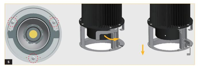
A. Screw the three indicated areasB. Lock the frameholder to the ceiling to hold the weight in place.
