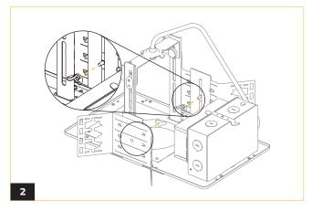
Secure the butterfly bracket by screwing in the provided wing nut.
