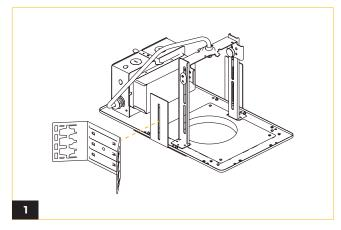
Align and attach the butterfly bracket to the side rail.
