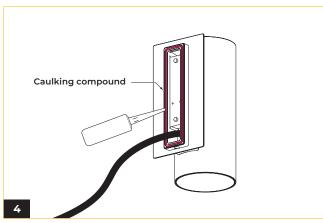
Apply silicone-based caulking compound along the perimeter of the mounting plate.
