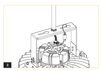
Clasp safety cable onto allocated slots on fixture bracket mount.
