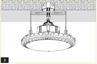
Make electrical connections between junction box and fixture according to the wiring diagram.
