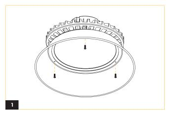
Install the Aluminum Shroud to the fixture with 3 supplied screws.
