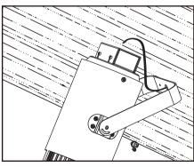
Attach the Yoke Mount bracket firmly onto the desired surface and secure it in place.
