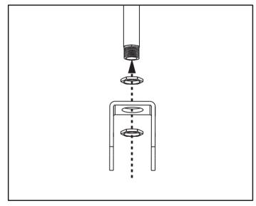
Fasten 2 Hex screw on either side of the uplight bracket.
