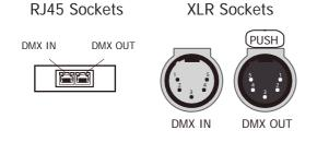
CONNECTION 5-PIN XLR RJ45 (CAT5e) Common WHITE/BROWN(PIN7) & BROWN(PIN 8) PIN 1 ORANGE(PIN 2) Signal -PIN 2 Signal+ WHITE/ORANGE(PIN 1) PIN 3 Spare \_ PIN 4 -Spare PIN 5
