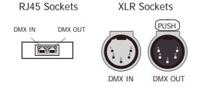
CONNECTION 5-PIN XLR RJ45 (CAT5e) Common WHITE/BROWN(PIN7) & BROWN(PIN 8) PIN 1 ORANGE(PIN 2) Signal -PIN 2 Signal+ WHITE/ORANGE(PIN 1) PIN 3 Spare \_ PIN 4 -Spare PIN 5
