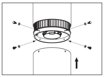
$\begin{array}{l} \textbf{Step 1} \\ \textbf{Bring up the diffuser to the fixture and align it to the indicated} \\ \textbf{openings and fasten in place with 4 thumb screws.} \end{array}$
