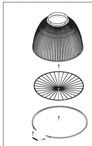
When specifying the conical lens accessory. Cover the shroud with the conical lens plate and fasten in place using the provided metal band.
