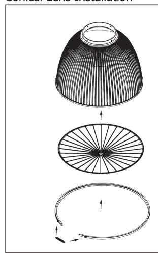
When specifying the conical lens accessory. Cover the shroud with the conical lens plate and fasten it in place.
