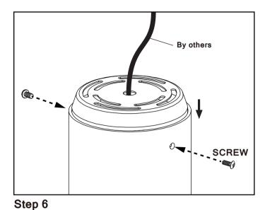
Fasten the lid and then Screw both sides of the fixture.
