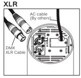
Connect DMX by using a standard shielded CAT5/6 cable
