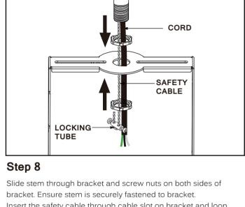
Insert the safety cable through cable slot on bracket and loop the cable using locking tube on the other side of stem and tighten the screws.
